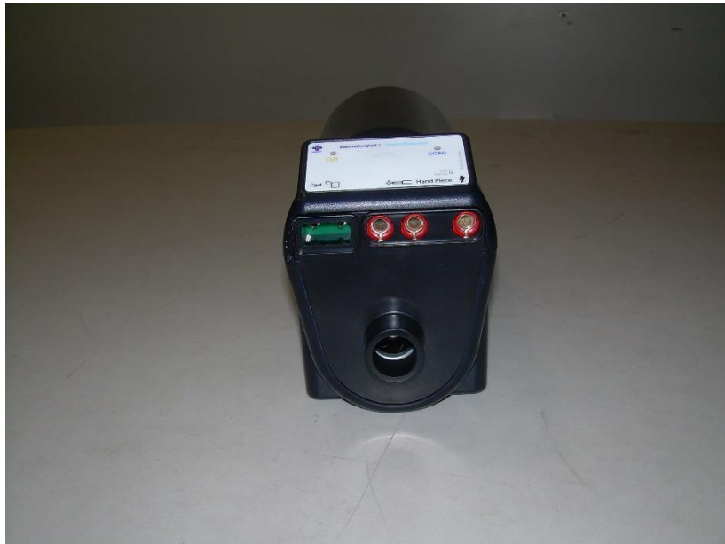
Photograph 4 – Side View of the EUT Showing Ports for Connection of the Hand Piece and Pad
