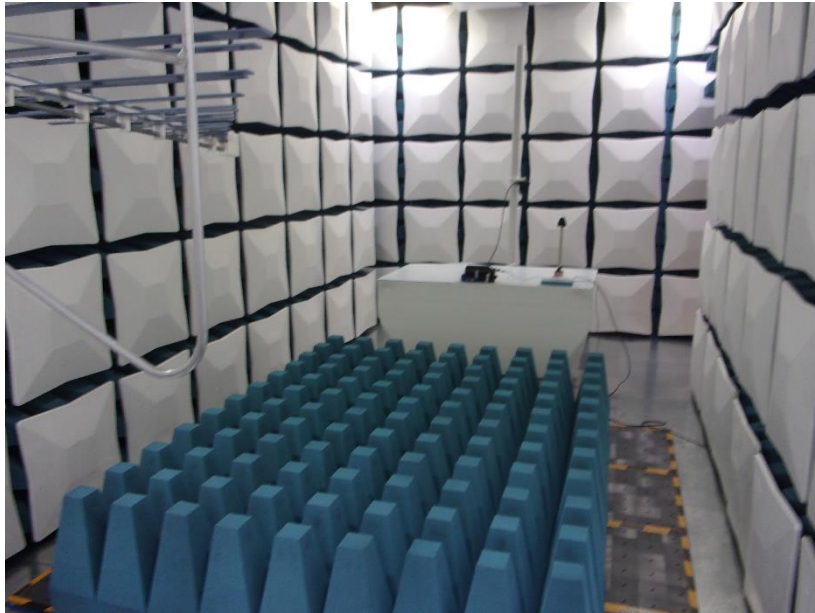
Photograph 13 – RF Immunity Test Setup Front
