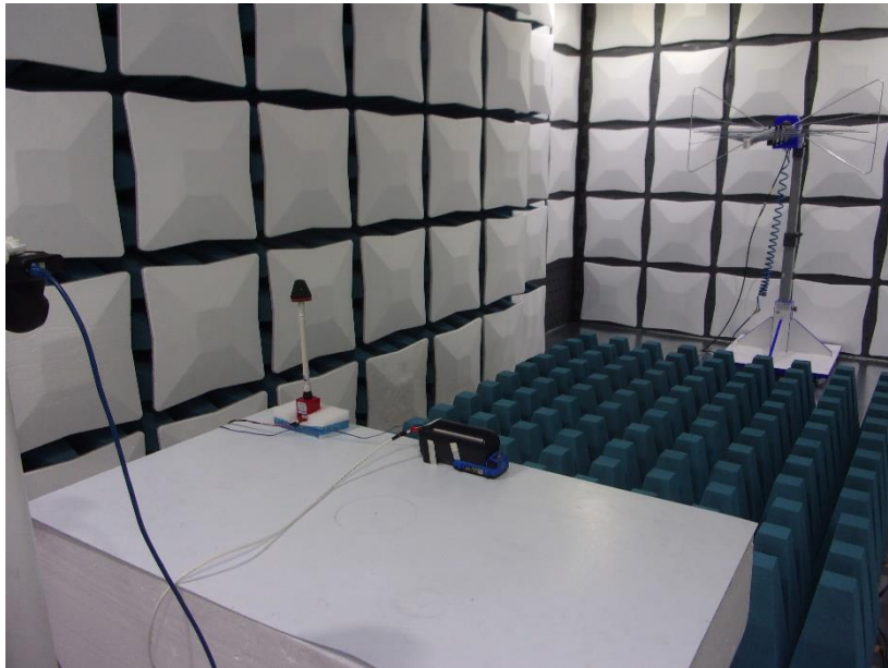
Photograph 14 – RF Immunity Test Setup Back
