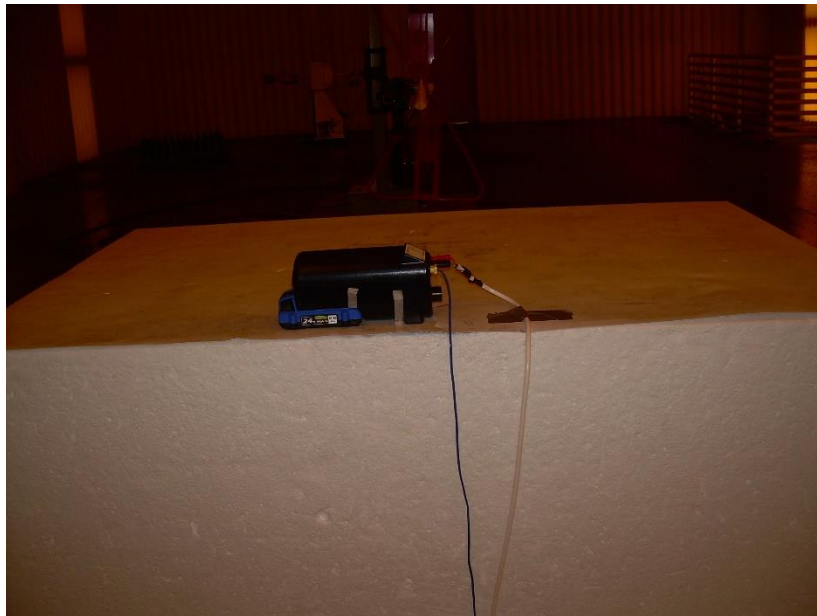
Photograph 2: Back View Radiated Emissions Worst Case Configuration
