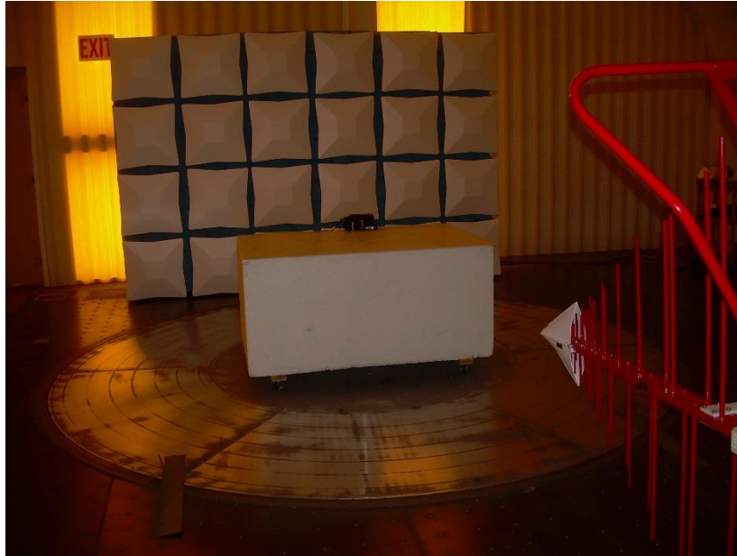
Photograph 1: Front View Radiated Emissions Worst Case Configuration
