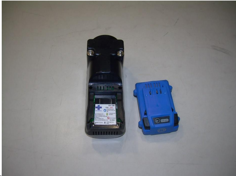
Photograph 7 – View of the Battery and Battery Port on the ESU-110
